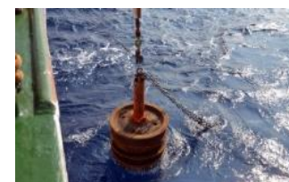
錨碇重錘 (廢鐵輪)
